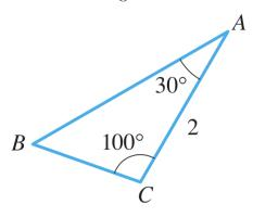
36. A tunnel is to be built through a mountain. A surveyor makes the measurements as shown in the figure. Use the surveyors data to estimate the length of the tunnel.
