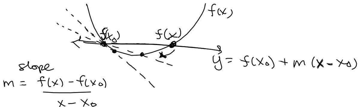
As  $x \rightarrow x_0$ , the secant line approaches the tangent line
