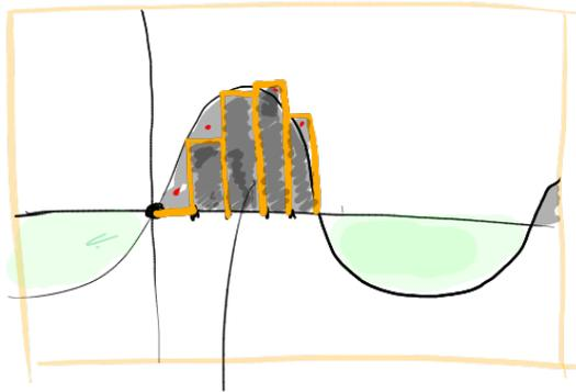
Each interval determines a rectangle, whose height is determined by a choice (left/right/midpoint) of the function.
